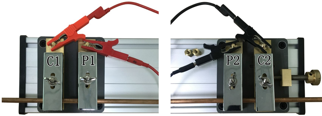
▲ connection diagram with TXJ-150 clamp
