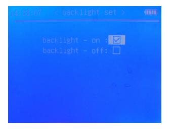
Backlight setting can turn on or turn off the backlight of the screen. When the lighting is insufficient or the screen display is too dim, it is better to turn on the backlight. Use ' $\uparrow$ ' or ' $\downarrow$ ' key to select the option then press 'OK' key to save the setting. The setting will be effective
