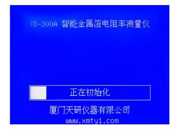
The full warming-up time for initialization is 5 minutes. After completion, it automatically enters 'measurement main interface'. During initialization period, if one wants to skip warming up and enter the measurement main interface directly, one can press measuring key "MEAS' once.
